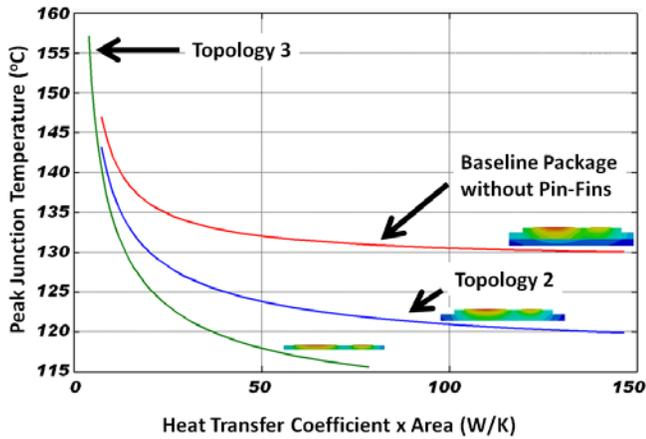
Figure 10. Thermal Performance by Heat Transfer Times Area
