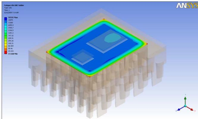
Figure 11. IGBT Solder Fatigue Life for Topology 1
