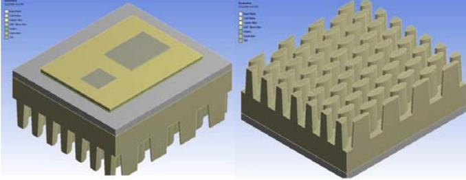
Figure 2. Topology 1: Baseline Package with Pin-Fin Cooling
