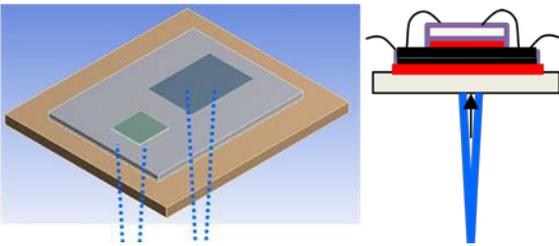
Figure 4. Topology 2: Indirect Jet Impingement on Base-Plate
