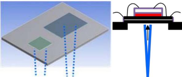
Figure 5. Topology 3: Indirect Jet Impingement on DBC Substrate
