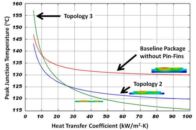
Figure 9. Thermal Performance by Heat Transfer Coefficient
