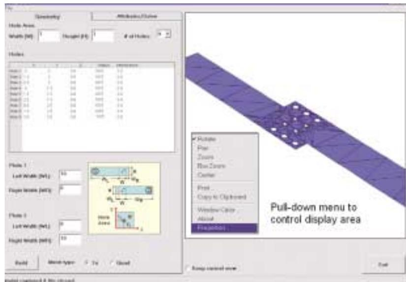
StressCheck from ESRD can be used as a "black-box" solver to analyze general problems such as fastened joints and stiffened panels. Users identify the number of holes in the joint or number of ribs in a stiffened panel, their locations, and a few dimensions. The handbook approach would need separate models for each design configuration.
