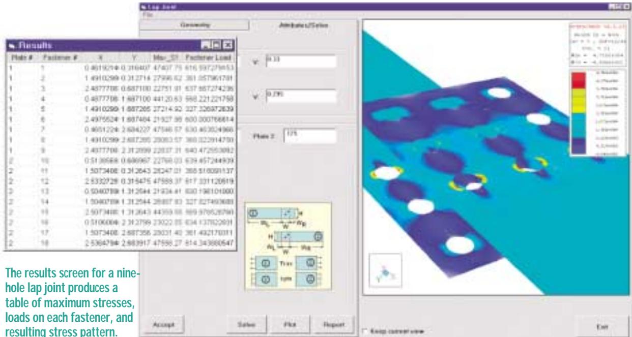
The results screen for a nine-hole lap joint produces a table of maximum stresses, loads on each fastener, and resulting stress pattern.
