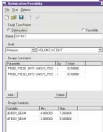
A dialog box from PTC's Behavioral modeling extension shows the optimization setup with a goal of minimum weight. The lower portion shows design variables and their limits for a box beam. Optimization is easily substituted for a sensitivity study that determines and plots effects of any Pro/E design variable to the natural frequency, or the probability of failure.
